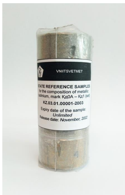
Fig. 2. State reference materials for the composition of metallic cadmium mark Kд0A-Kд1 (set) KZ.03.01.00001-2003 (IRS 0633:2004)
