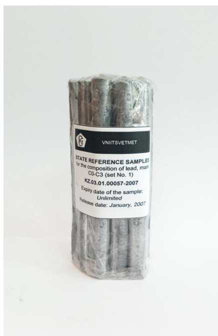
Fig.1. State reference materials for the composition of lead mark C0-C3 (set No. 1) KZ.03.01.00057-2007
