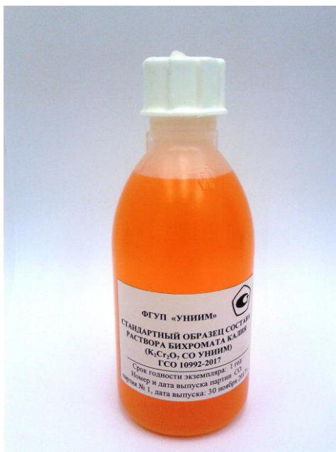
Fig. 1 . The appearance of the CRM unit of 0,1 M potassium dichromate solution
