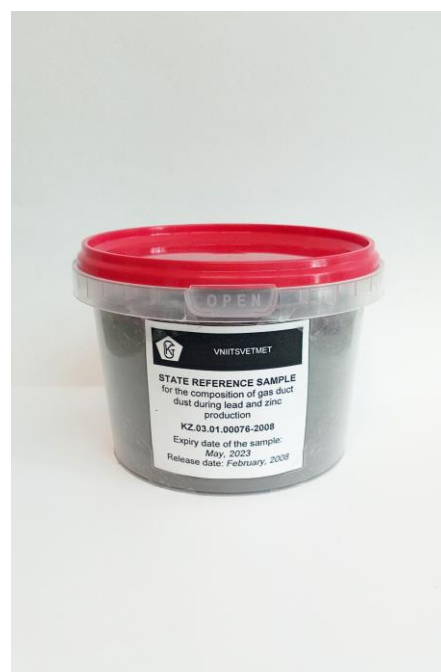
Fig. 3. State reference material for the composition of gas duct dust during lead and zinc production KZ.03.01.00076-2008 (the COOMET CRM 0062-2008-KZ)
