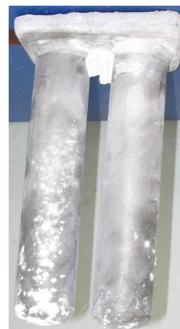
Figure 4. Billets of Ni alloy CRM obtained by directed crystallization [3]
